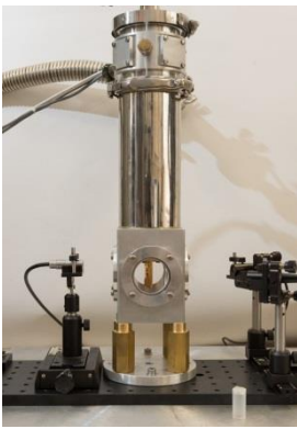
Continuous flow optical cryostat for 4÷300 K temperature range
